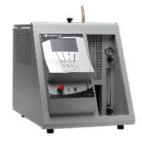
Fully automatic and easy to use, the NMC 445 provides all safety requirements for a carbon residue measurement of carbon residue formed after evaporation and pyrolysis of petroleum products. It offers you the best specifications thanks to an automatic calculation of carbon residue % (Required balance).
